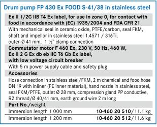
When using the pump with hose and hand nozzle, the flow rate is max. 60 l/min.\*, viscosity max. 1 200 mPas, delivery head max. 9 mwc.
