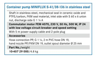
When using the pump with hose and hand nozzle, the flow rate is max. 60 l/min.\*, viscosity max. 1 000 mPas, delivery head max. 9 mwc.
