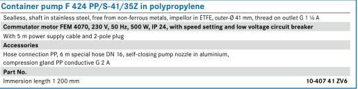
When using the pump with hose and hand nozzle, the flow rate is max. 35 l/min.\*, viscosity max. 800 mPas, delivery head max. 18 mwc.
